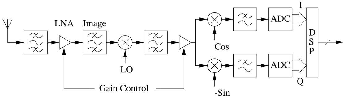
Figure 3: Traditional heterodyne receiver architecture based on the parallel data detector concept.
