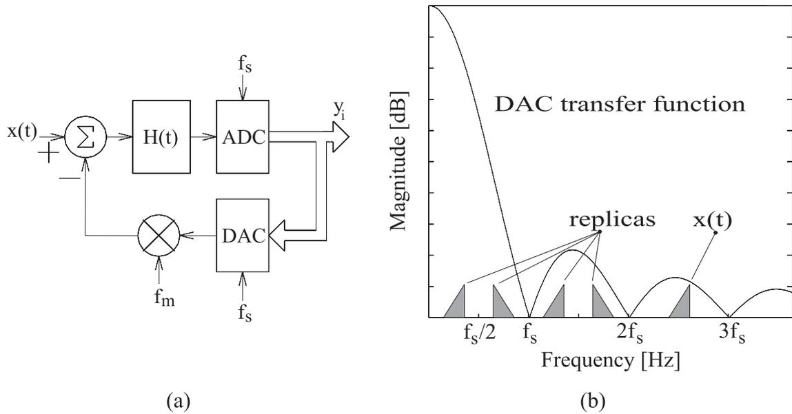
Figure 10: Sub-Sampling bandpass delta-sigma converter [14]. (a) Structure of the circuit. (b) Frequency domain signal representation.
