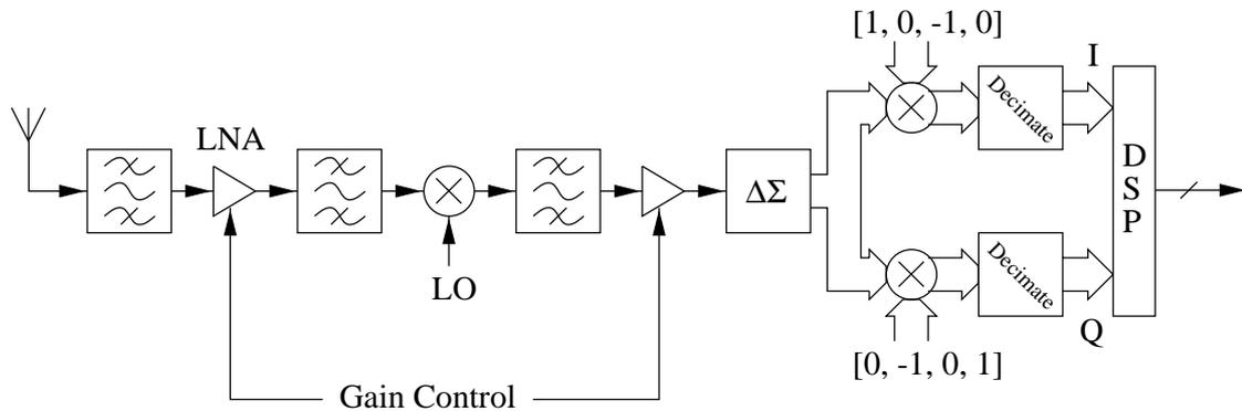
Figure 8: Low-IF receiver architecture based on bandpass delta-sigma conversion.
