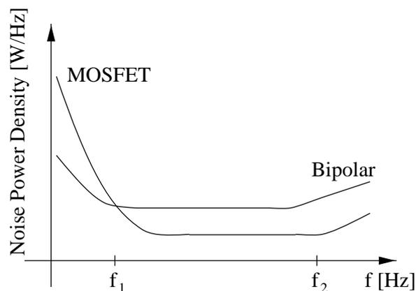
Figure 5: Sketch of Noise Power Spectral Density characteristics of MOSFET and BJT's. The frequencies  $f_1$  and  $f_2$  are typical of the order kHz and several hundreds MHz, respectively [16].
