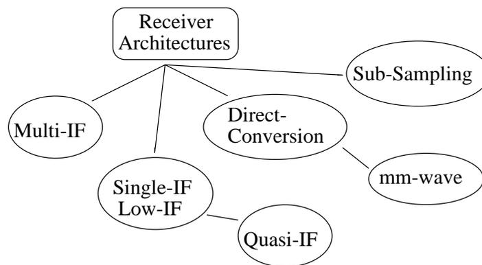
Figure 2: Architecture relation diagram presenting the most common architectures, their relations, and also a few novel architectures.
