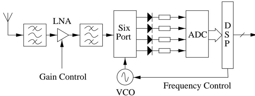
Figure 11: Millimeter-wave receiver architecture [26].
