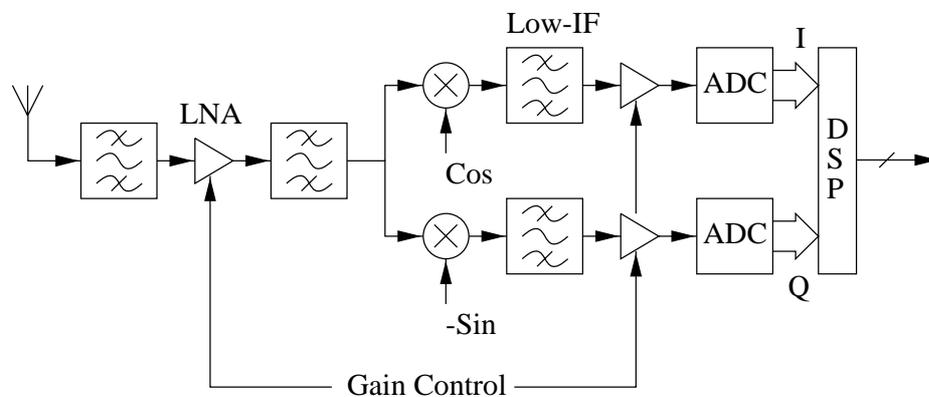
Figure 6: Low-IF receiver architecture.
