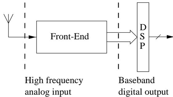
Figure 1: Front-End interface definition. The front-end accepts a high frequency antenna signal and delivers a Nyquist rate digital baseband output to a subsequent DSP unit.
