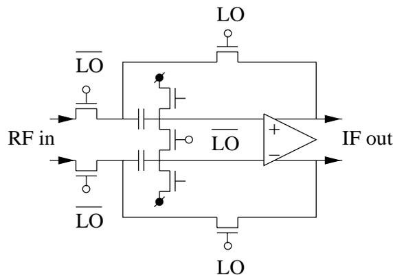
Figure 9: UCLA sub-sampling track-and-hold mixer implementation [3].
