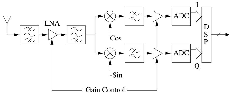
Figure 4: Direct-conversion receiver architecture.
